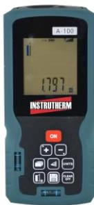
**TRENA A LASER MOD. TR-100 ESCALA DE 0.03 A 100M, CÁLCULO DE ÁREA, VOLUME E MEDIÇÃO INDIRETA**
